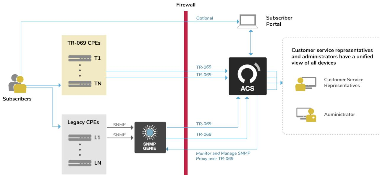
Figure 1. The addition of SNMP Genie to the Incognito Digital Home Experience solution extends TR-069 support to legacy devices
